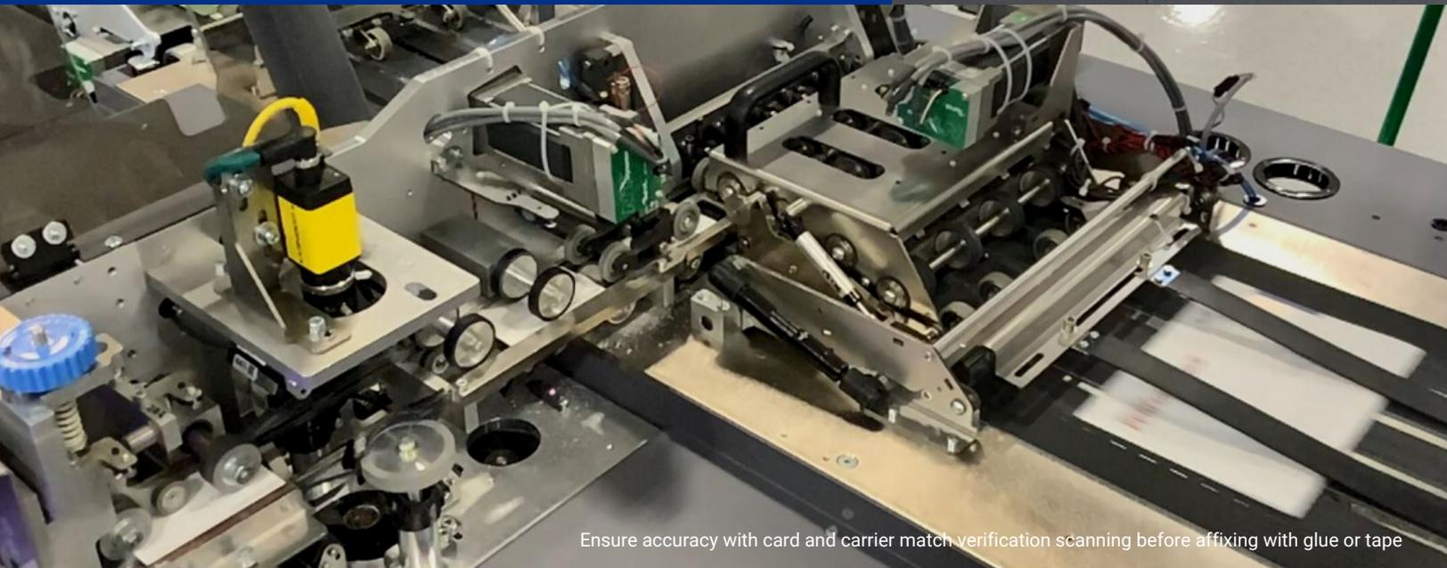
Ensure accuracy with card and carrier match verification scanning before affixing with glue or tape
