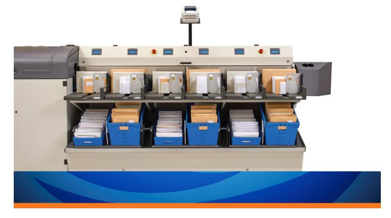
The Mixed Mail Stacker (MMS) solution is made up of a single or double-sided configuration. It consists of 6 pocket increments per stacker, a control system and mail stack mechanical hardware capability that can process up to 10mm thick mail. The MMS has a single-side, optional double-side, and turn-around module to support technology flexibility and Vantage™ front-end configurations based on current or future business needs.
